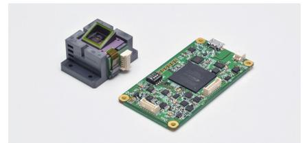
Driver circuit for MEMS mirror C15087
